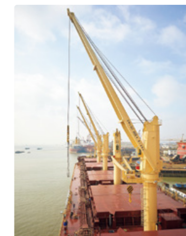
Electric Crane (36t)
