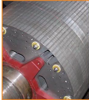
PM segments embedded inside the rotor structure
