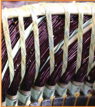
Three separate winding groups
